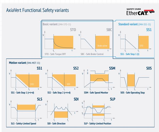
The Basic variant (SMA-STO-11) includes Safe Torque Off (STO) and Safe Brake Control (SBC), while the Standard variant (SMA-SS1-11) introduces also SS1-t (Safe Stop 1 with time monitoring) reducing the necessity for an external Functional Safety switch.
