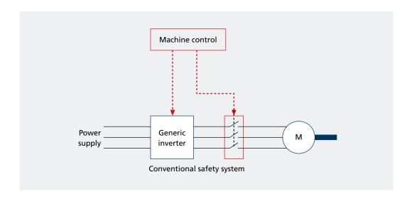
Bonfiglioli has integrated the Safe-Torque-Off system (STO, EN61800-5-2) in Agile inverters to reduce the size of control panels, minimise the number of operating components, simplify control, and eliminate the mechanical stress caused by the sudden application of the brake while the shaft is still turning. In an emergency this system disconnects the motor in compliance with EN13849-1 PL d and EN61508 SIL2, without the need for external contactor.
