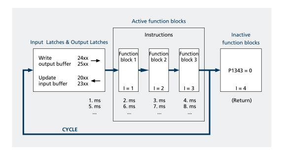
As in any control panel PLC, cycle management is entrusted to the operating system and is independent of all other processes managed by the CPU.
