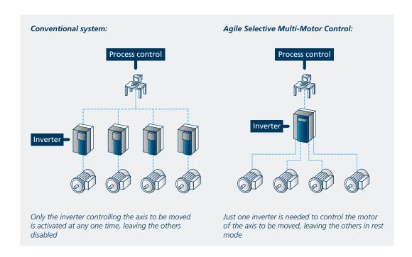
By using two digital inputs in binary combination mode, users can activate the inverter's parameter configuration corresponding to just one of the four motors, thus excluding the other three.
