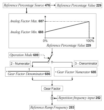
Signal flow diagram for scaling the gear factor via the reference percentage source:
