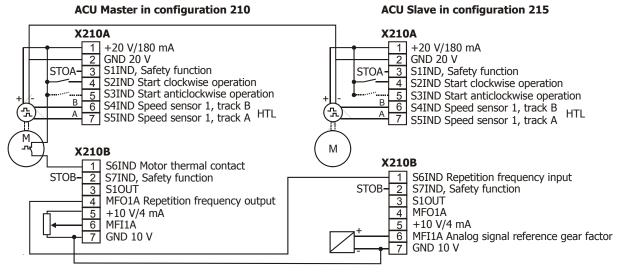
To ensure correct operation, connect the GND terminals between the frequency inverters.
