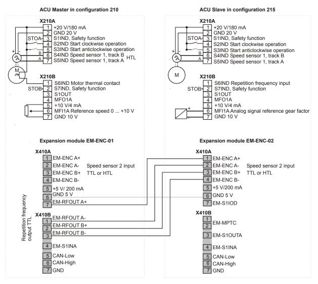
The digital inputs of the frequency inverter or the speed sensor inputs EM-ENC (extended speed sensor evaluation) can be used alternatively as speed sensor inputs.
