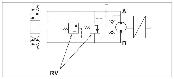
RV = pressure relief valves calibrated to pRV < pmax.
