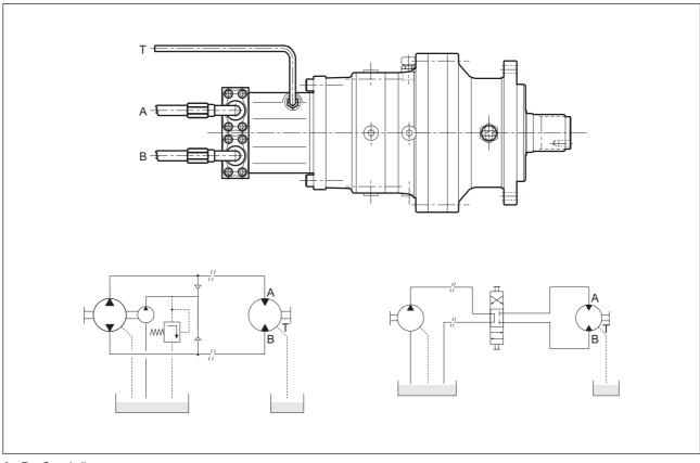
**A - B** = Supply lines **T** = Drainage
