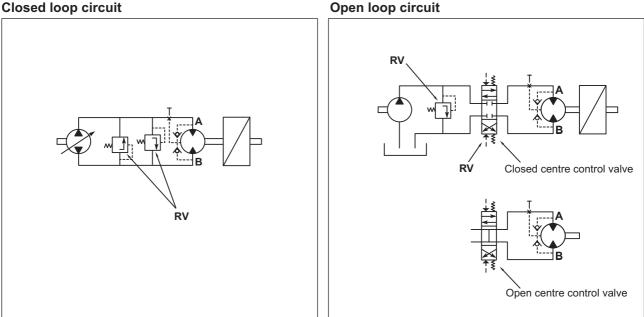
RV = pressure relief valves calibrated to pRV < pmax.
