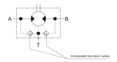
If the drain port is connected up, pressure at the shaft seal is always equal to the pressure in the drain line.
