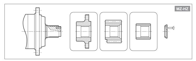
Always use the stop end plate supplied with the gear unit.
