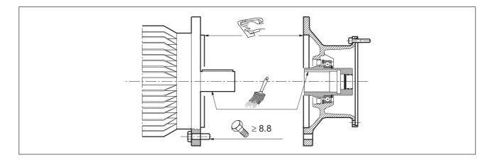
Provided all the above checks have been performed and passed and all other instructions in this manual have been strictly observed, an electric motor with ATEX rating equal to or greater than that of the gear unit may be installed, thus forming a gearmotor which itself complies with the provisions of Directive 94/9/EC.
