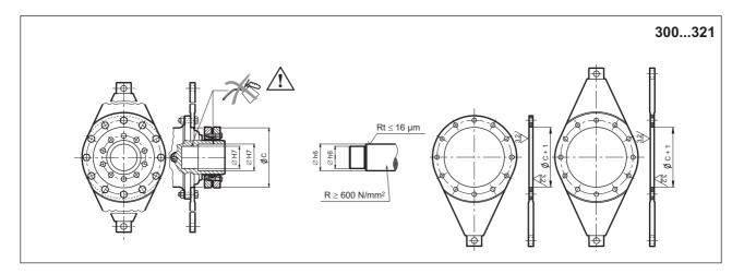
Do not use molybdenum bisulphide or any other grease, which could reduce the friction of the mating surfaces and affect the performance of the shrink disk.
