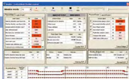
Universal monitor with recording/reproducing capability
