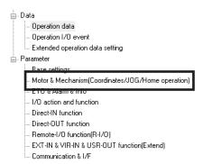
Change the "Motor rotation direction" parameter to "Positive side=counterclockwise (the driver parameter is applied)" or "Positive side=clockwise (the driver parameter is applied)."
