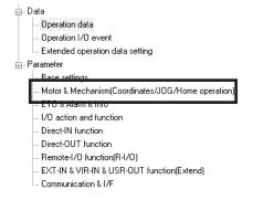
3. Change the "Initial coordinate generation & wrap coordinate setting" parameter to "Manual setting."
