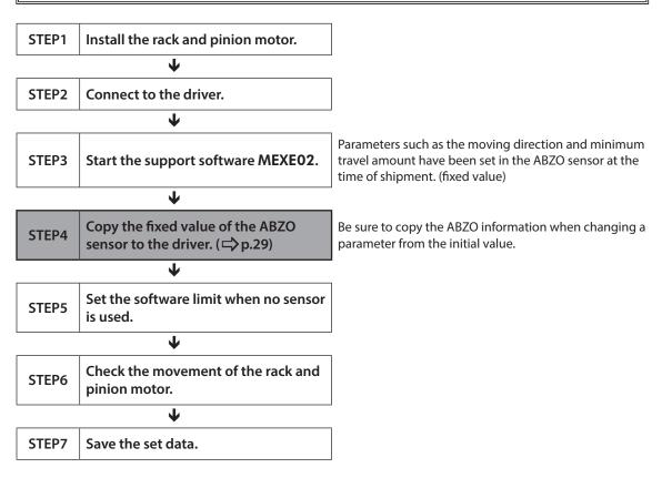
For some parameters, the unit of travel amount may change from "mm" to "step" if the parameter is changed from the initial value. Note that the unit of travel amount cannot return to "mm" if it changed to "step."
