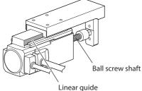
Linear guide (Apply grease to the opposite side as well)
