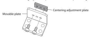
2. Secure the movable plate to the guide block using screws.
