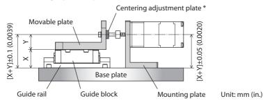
\* It is used when the accuracy of component parts is not enough to perform centering. Also, it is used when the stacking tolerance of parts is adjusted.
