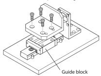
3. Move the movable plate closer to the mounting plate, and check that there is no gap between the plates.
