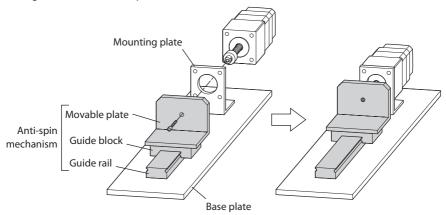
With the non-guide type actuator, the customer is required to perform centering between the actuator and anti-spin mechanism. The installation method varies depending on whether the component parts of anti-spin mechanism have an accuracy that centering can be performed. If the component parts does not have enough accuracy to perform centering, jigs (centering shaft, centering adjustment plate) are needed.
