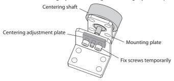
5. Slide the movable plate to check that it moves smoothly, and tighten the screws on the centering adjustment plate.
