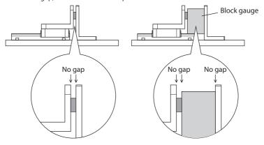
4. Using the centering shaft to resemble the actuator, insert the centering shaft to the mounting plate.
