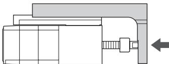
2. The set collar (stopper) presses against the pilot section, and the TLC output is turned ON.
