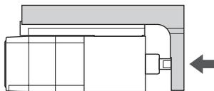
3. The ball screw shaft reverses and stops after moved according to the value set in the "(HOME) Backward steps after first entry in push-home-seeking." (factory setting: 0)
