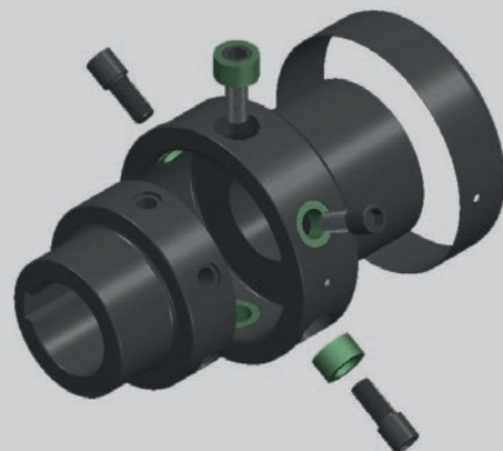
Exploded diagram of compact elastic coupling
