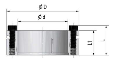
Medium torque capacity Self-locking & self-centering Axial fixation of hub during tightening: no Max tolerances: shaft h8; hub bore H8 Shaft / hub bore surface finish:  $0.8 \le Ra \le 3.2 \ \mu m$  From size 55 x 85 and above: rings NOT SLIT
