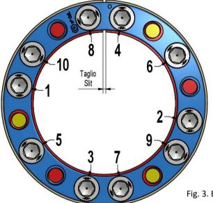
Fig. 3. Example of tightening pattern.
