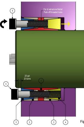
Fig. 4. Release of rear thrust ring.
