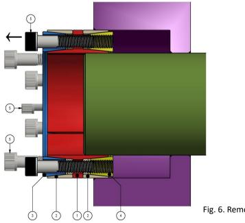
Fig. 6. Removal of Locking Assembly.
