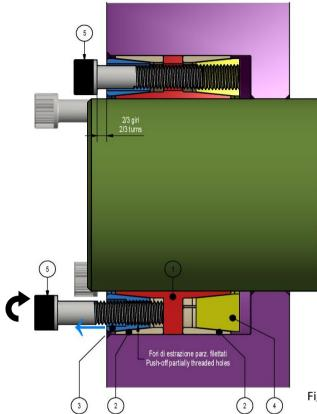
Fig. 5. Release of front thrust ring.
