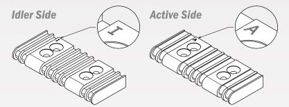
Movex 530 Pro LBP Nosebars are special Nosebars, specific to optimize the characteristics of this particular belt. It can be installed in two different ways: idler side and active side, depending if you want to obtain the accumulation or acceleration effects of the goods. In both modalities the same Nosebar is used: it simply needs to be installed on one side rather than the other. One face of the Nosebar is set up for the accumulation function and the opposite one for the acceleration function.
