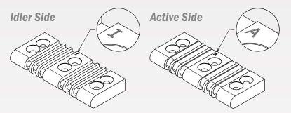
Movex 530 LBP Nosebars are special Nosebars, specific to optimize the characteristics of this particular belt. It can be installed in two different ways: idler side and active side, depending if you want to obtain the accumulation or acceleration effects of the goods. In both modalities the same Nosebar is used: it simply needs to be installed on one side rather than the other. One face of the Nosebar is set up for the accumulation function and the opposite one for the acceleration function.
