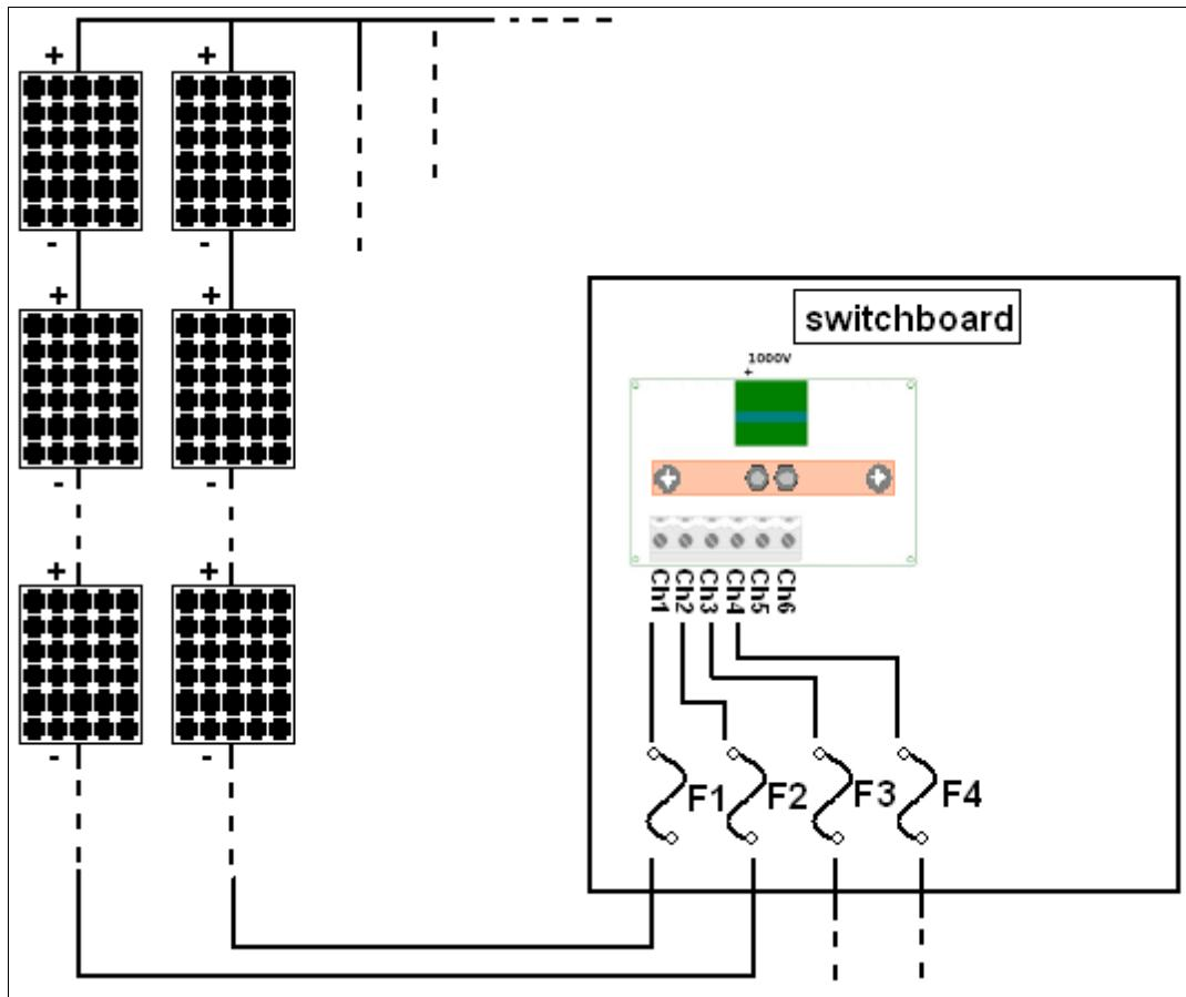
Each channel can read a maximum current of 30A (although typically the current of each string is more or less 7 ÷ 8A). After the strings input connector, on the ST1 board there are two resistors in parallel, they are necessary to detect the current flow:
