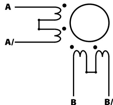
Wiring diagram of a 8-wire stepper motor connected in bipolar series to the drive phases.
