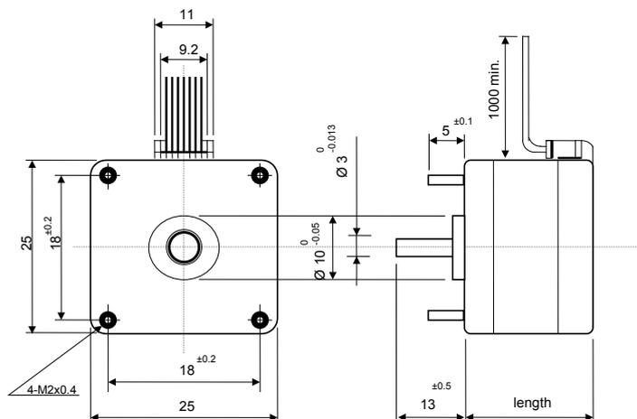
2-phases permanent magnet step motors
