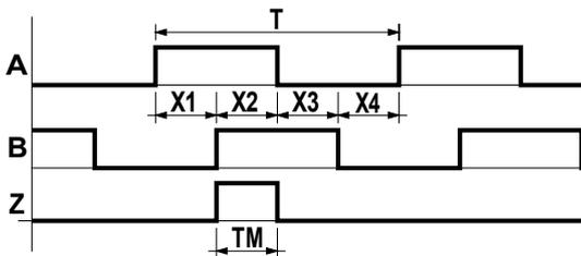
The waveforms viewed from the coupled plate and clockwise rotation
