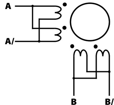
Wiring diagram of a 8-wire stepper motor connected in bipolar parallel to the drive phases.
