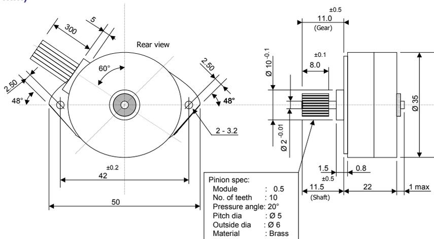
2-phases permanent magnet step motors
