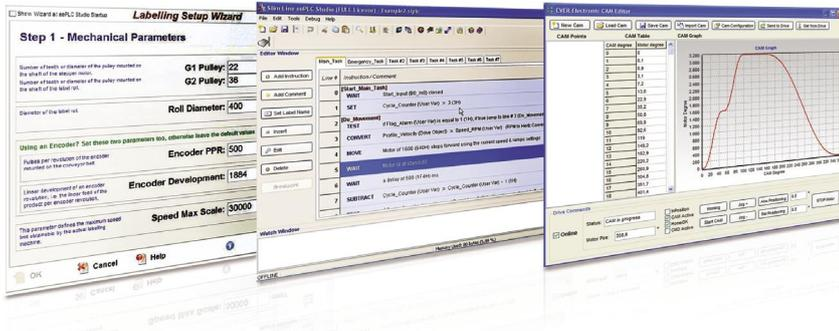
The eePLC Studio programming environment is provided with a wizard, namely guided procedures to write in just a few steps the programme for simple or complex axis automation. Among the available wizards there are, for example: the complete control of a labelling head, axis control in an electronic cam, electric shaft tracking from master encoder or analog input, etc.
