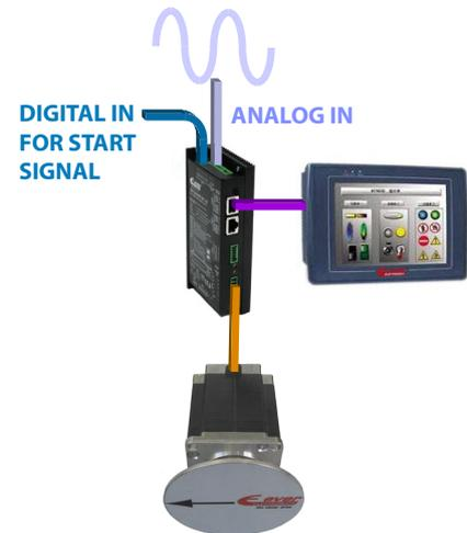
An intelligent positioning device with motion quotes and relative speed and acceleration profiles defined inside the drive. These profiles are obtained according to limit switch sensors and homing procedures. As an alternative, the motion profiles can be generated by external HMI or PLC.
