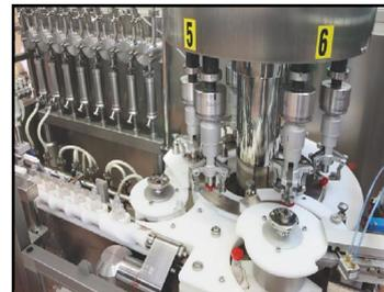
Thanks to stepper motor torque control, Ever Elettronica can offer innovative solutions for various processes management such as: corking, filling, encapsulating, etc. offering a great compromise between high performance and flexibility, which can be obtained using servo-brushless motors, as well as the saving deriving from the use of mechanical or pneumatic solutions.
