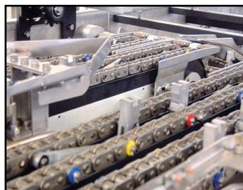
The format change process can be directly managed by PLC by means of quotes sent via fiellbus, or by selecting the quotes from a HMI device. It can be controlled in 'Stand Alone' mode using the programmable drive. Thanks to Ever Elettronica advanced drive techniques, it is possible to obtain speedy and precise format changes in both modes.
