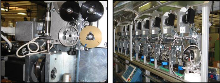
The solution for this kind of machines controls the wire advancement by means of a stepper motor driven in a closed loop, capable of adjusting the stability of the wire speed emission, checking the possible slide through an encoder and allowing a precise and repetitive working process.
